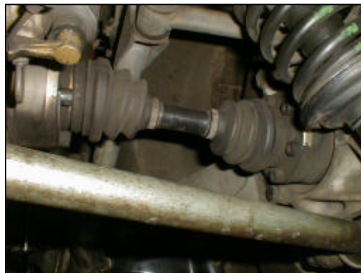
The driveshaft. Note the allen-head capscrews on each end. Inspect the rubber boots carefully.
