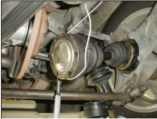
The inboard side of the axle wired out of harm's way. Rotor to left.
