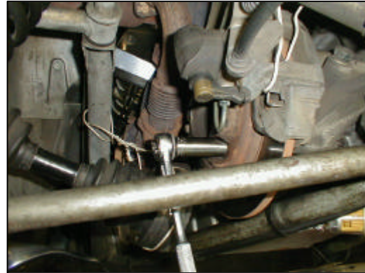
Note the caliper wired out of the way, now the rotor nuts are fully removed.
