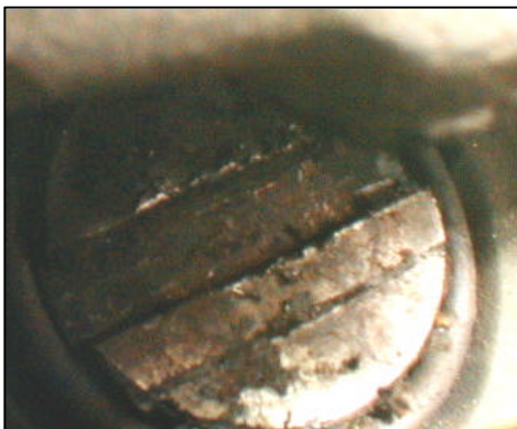
Close-up of the face of the brake caliper. The middle slot is 1/4" wide, the line indicates the top of the caliper.
