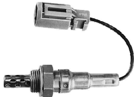
Typical Oxygen Sensor: May have up to four wires.
